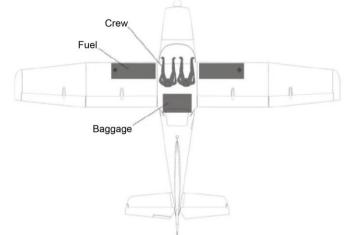
Aircraft C.G. = empty aircraft C.G. + crew increment on C.G. + fuel increment on C.G. + baggage increment on C.G.
