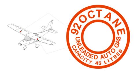
Around drain valves on the bottom side of the wings:
